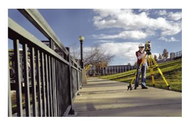
Long-range DR – hard-to-reach or unsafe targets can now be measured as easily as those measured with a prism.
